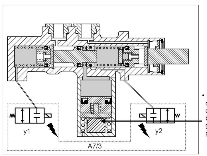
Further pedal travel causes piston to compress rubber
