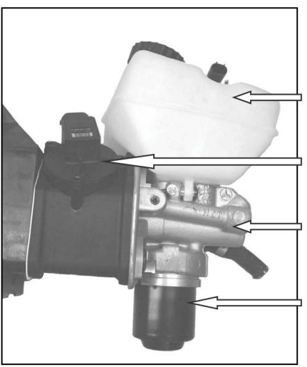
The Brake Operating Unit (BOU) consists of the following:
