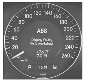
Complete ESP control module failure - Instrument cluster will scroll through failure displays
